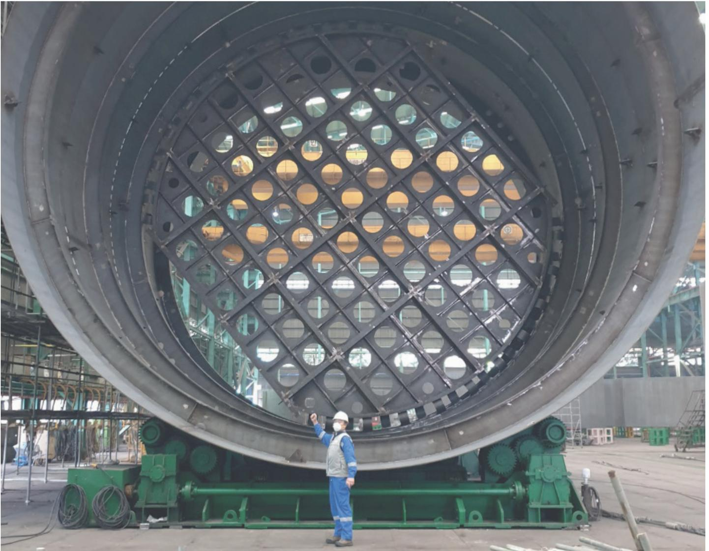
*Cryogenic LNG tank under construction in Korea*
