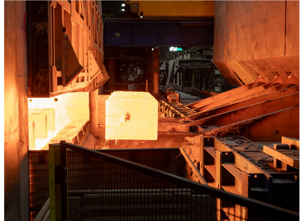
New Bloom Reheat Furnace at Faircrest Plant
