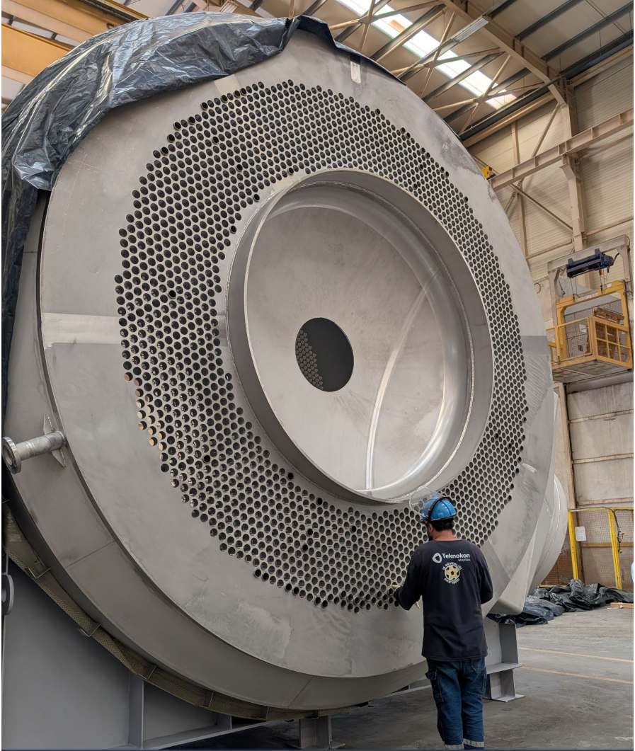
Cold Interpass Heat Exchanger
