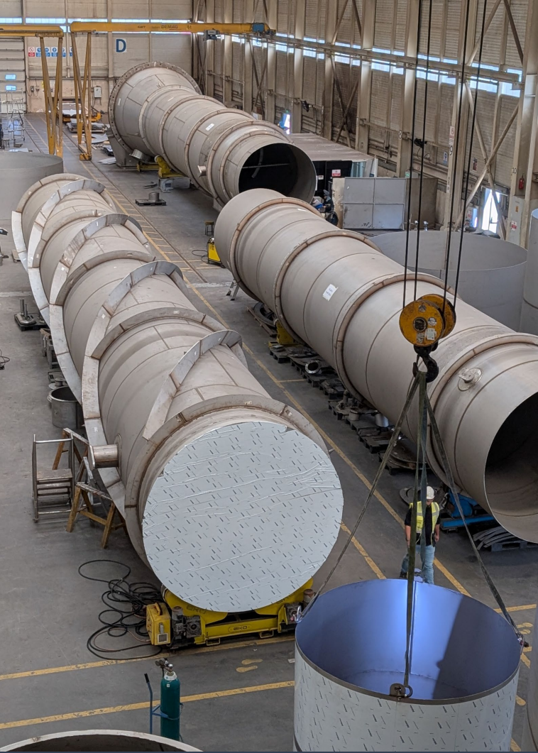
Duplex Plant Stack
