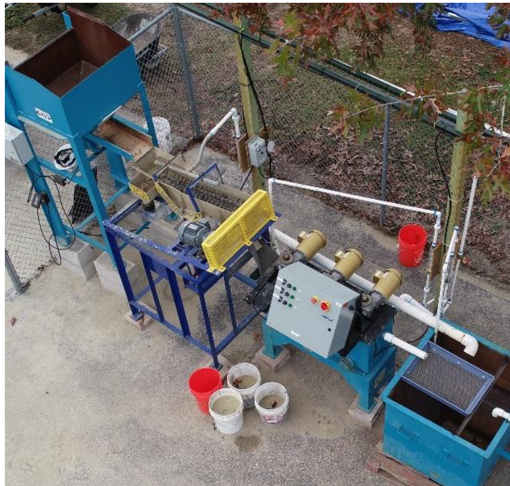
Figure 10-5 Primary Cyclone, Hydraulic Classifier and Dewatering Screen
