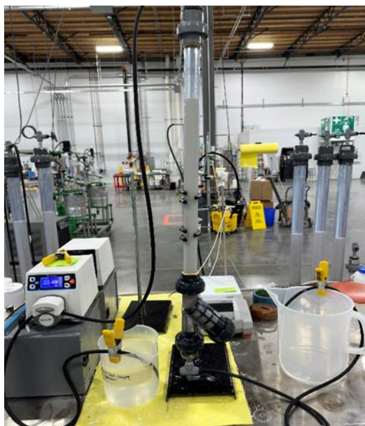
Figure 10-18 Bench Scale Ion Exchange Column Testing Apparatus
