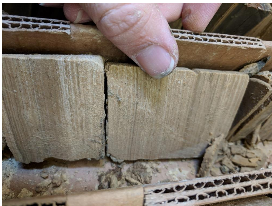
Figure 8-1 Half Core Sawed by a Diamond Blade
