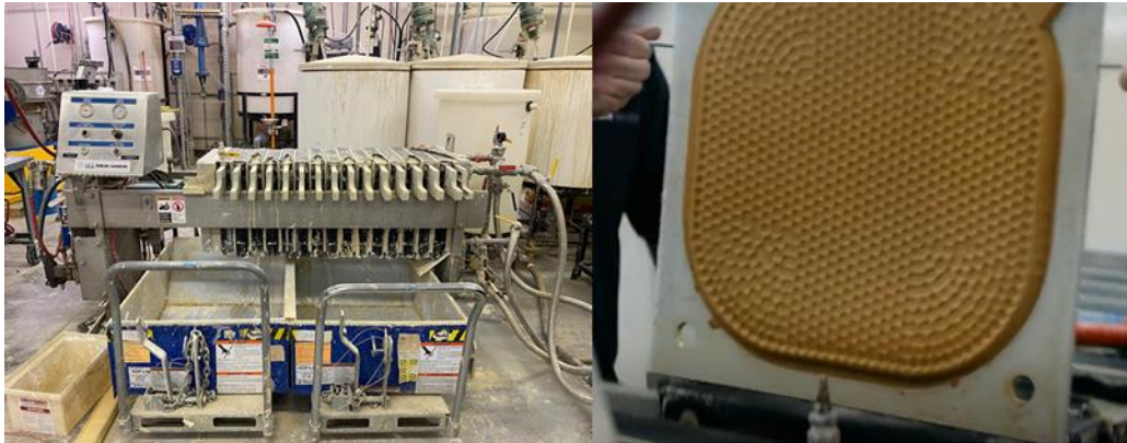
Figure 10-13 LAC Pilot Membrane Filter Press and Resultant Filter Cake
