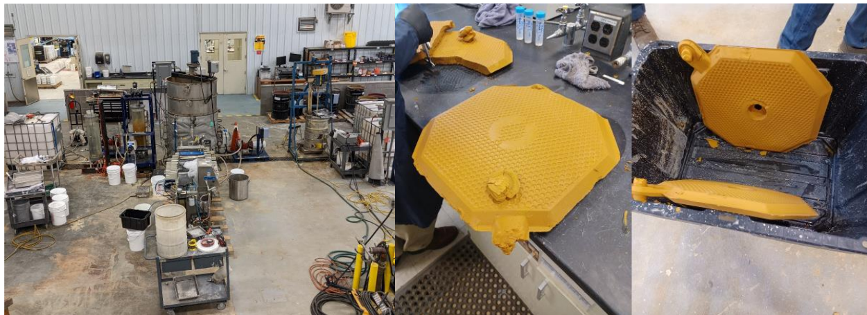
Figure 10-14 Pilot CCD and Filtration Setup and Resultant Filter Cake
