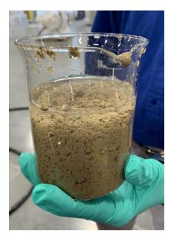
Key variables included pool depth, differential speed, polymer dosage, G-force, and feed rate. This test demonstrated that under optimized conditions, a cake dryness of 55 to 60 wt% solids could be achieved further confirming previous pilot results (Section 13.2.1.1). The machine performance during the pilot testing was used for key scale-up parameters.
