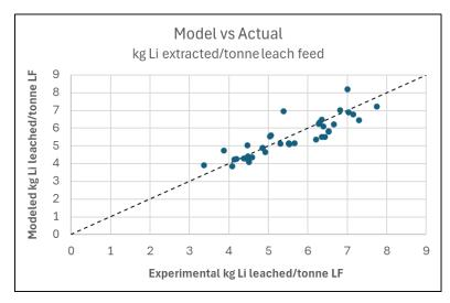
Generally, there is good agreement between the predicted values and data. On average over the 40 samples, the observed lithium extraction was 2% higher than the predicted value. Note that a strong correlation between leach feed composition and residual acid was also found.
