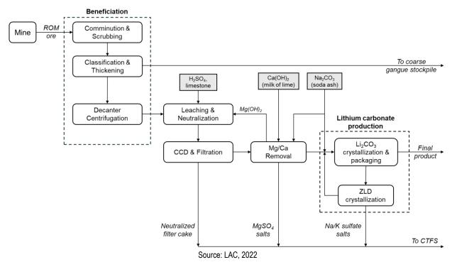
In beneficiation, ROM ore is crushed then mixed with water and fed to unit operations designed to liberate lithium bearing clay from gangue material. The clay is separated from coarse gangue in classification, with coarse gangue being stockpiled and eventually used as pit backfill material. The clay fines are then sent to the first dewatering stage (thickening) followed by decanter centrifuging (Figure 17-2).
