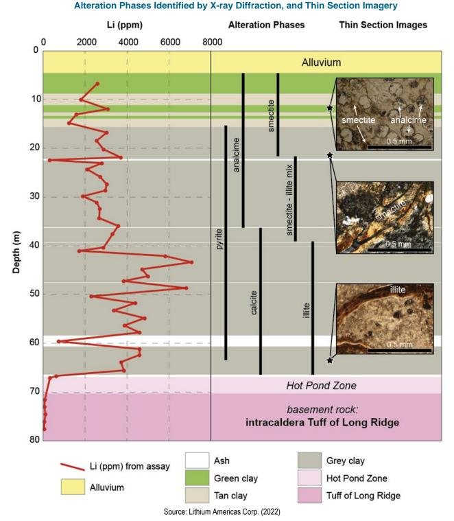
Most of the moat sedimentary rocks drilled in the Thacker Pass basin contain high levels of lithium (>1,000 ppm). Intervals that consist mostly of ash or volcanic rock have lithium contents of less than 800 ppm whereas intervals dominated by claystone contain more lithium (>1,000 ppm). Many intervals have very high lithium contents (>4,000 ppm). Intervals with extreme lithium contents (>8,000 ppm) occur sporadically in the Thacker Pass deposit.
