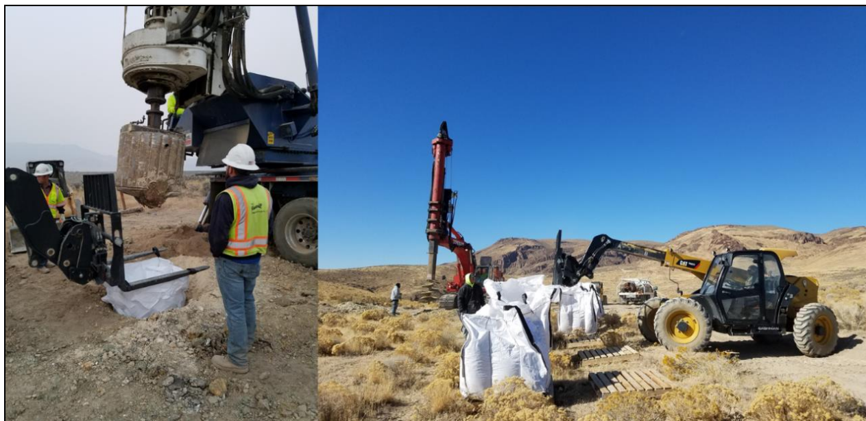
Figure 13-2 Bulk material sampling
