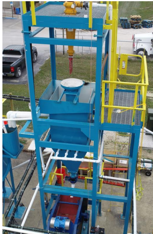
Figure 13-10 Primary Cyclone, Hydraulic Classifier and Dewatering Screen
