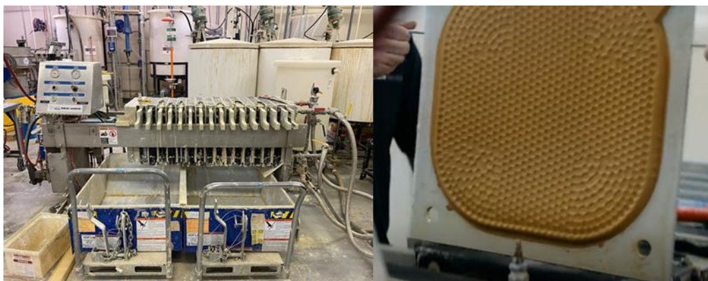
Figure 13-20 Pilot membrane filter press and resultant filter cake
