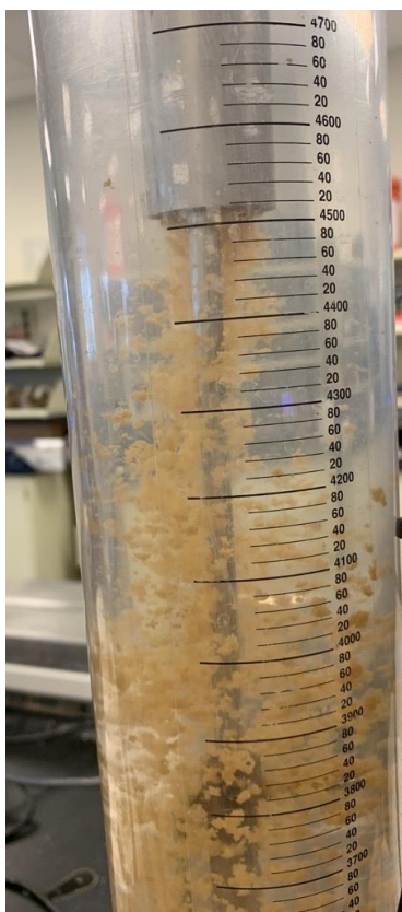
Figure 13-22 Dynamic Thickener Testing at FLSmidth
