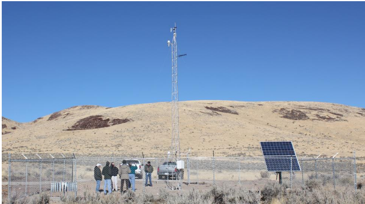
Figure 5-1 Photograph of the On-Site Meteorological Station, Including Tower, Solar Power Station, and Security Fence
