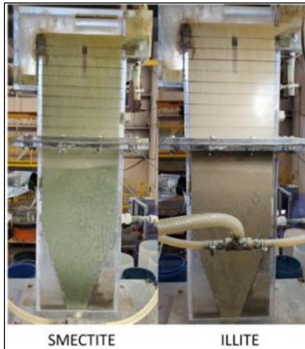
Figure 13-5 Smectite and illite fines separation in a pilot crossflow separator
