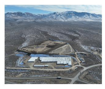
**Figure D:** Major earthworks completed to date include an initial box cut at the northwest corner of the plant location to de-risk the civil engineering program by giving us better data on the soil and geotechnical conditions. A second box cut has commenced.
