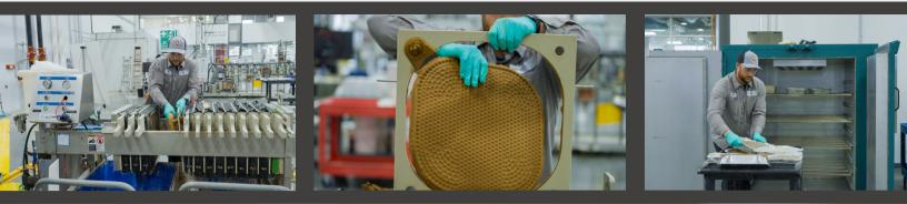
A pilot test was also conducted on a lithium carbonate dryer and cooler units, confirming performance and generating data to be used for industrial equipment selection. The dryer is used at the end of the process to ensure the lithium carbonate has a low moisture percentage, which is a battery grade requirement. The cooling step lowers the temperature of the final product as it exits the dryer prior to packaging.
