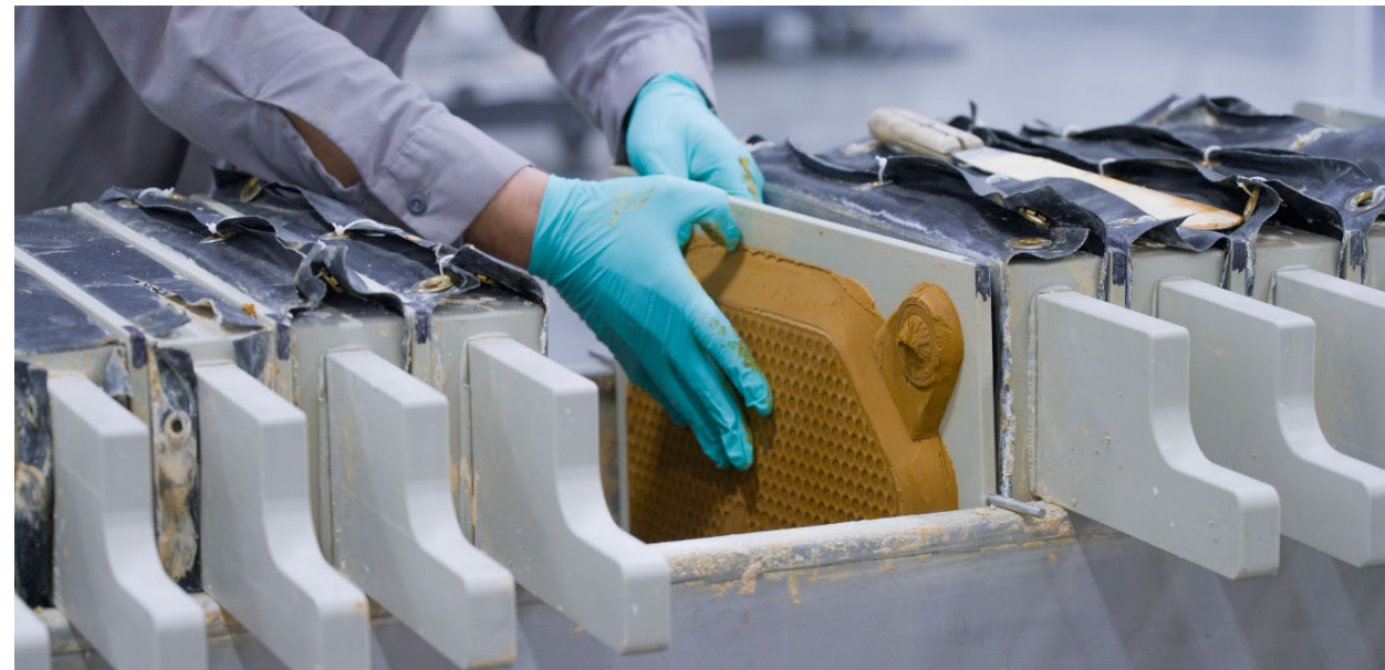
Neutralized clay tailings are pressed into filter cakes, maximizing water recycling efforts
