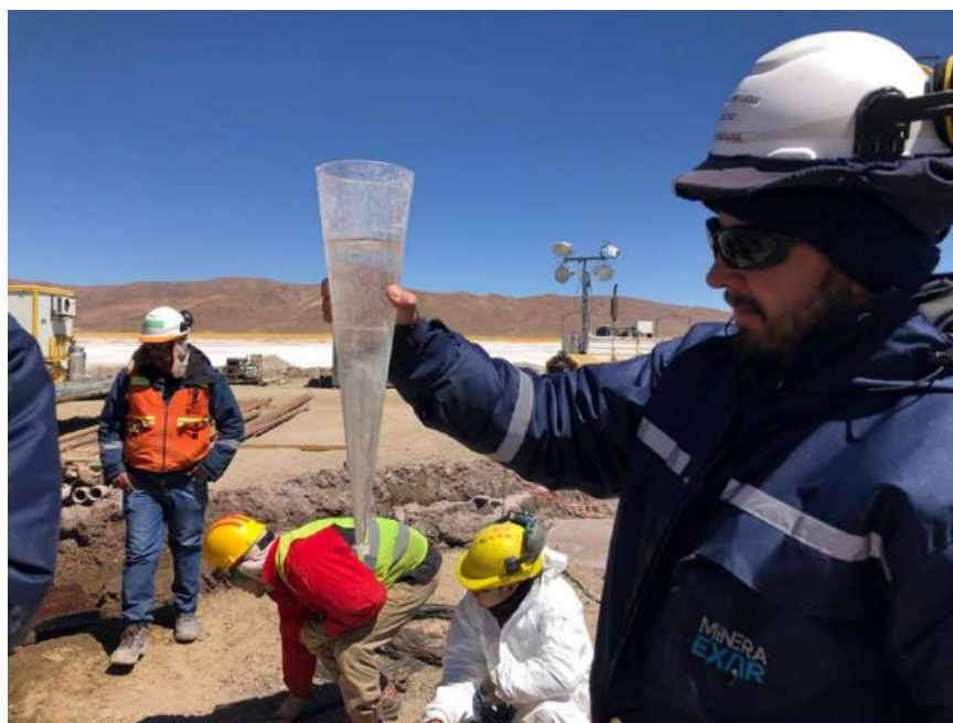
Figure 11.4 Measuring Sediment in an Imhoff Cone
