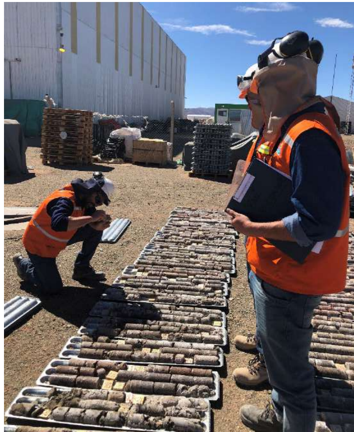
Figure 11.3 Collecting an Undisturbed Sample from Core
