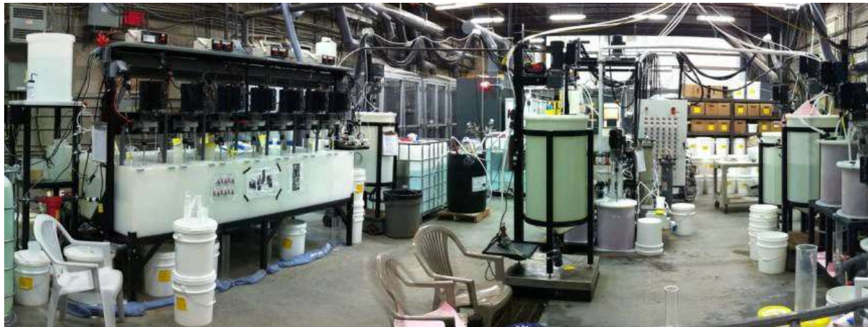
Figure 13.10 Pilot Plant (SX-Purification-Carbonation-Filtration-Washing Pulp)
