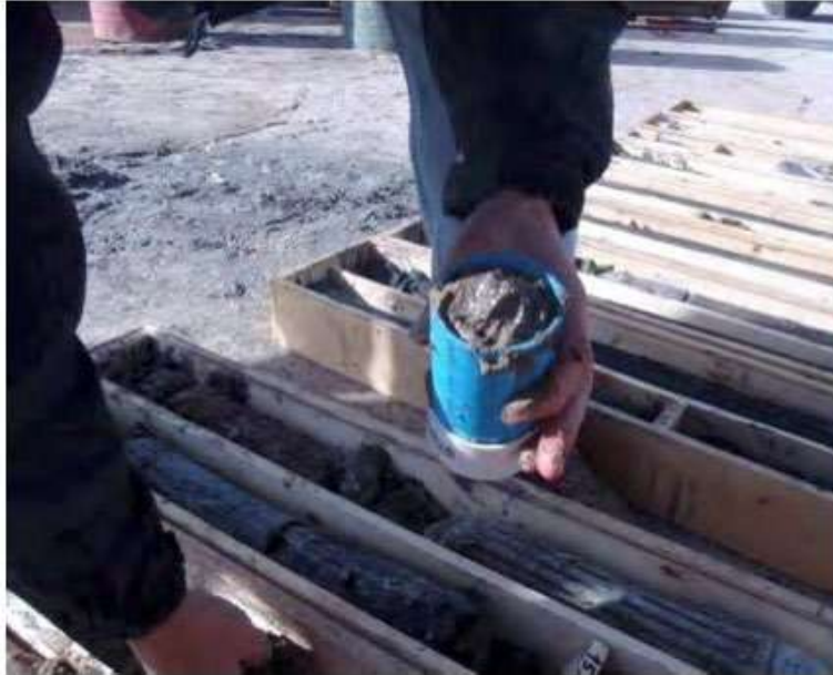
Figure 11.2 Collecting an Undisturbed Sample
