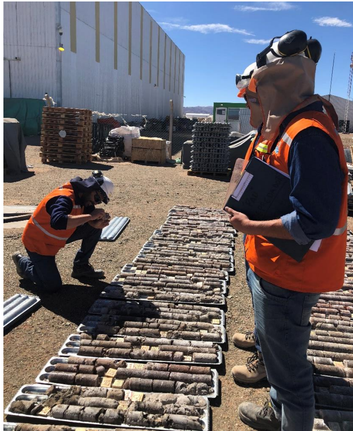
Figure 11.3 Collecting an Undisturbed Sample from Core
