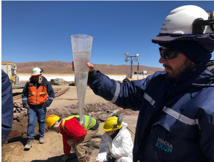
Figure 11.4 Measuring Sediment in an Imhoff Cone
