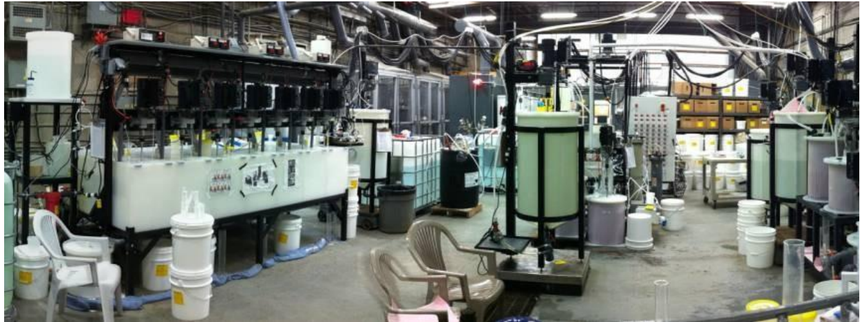
Figure 13.10 Pilot Plant (SX-Purification-Carbonation-Filtration-Washing Pulp)
