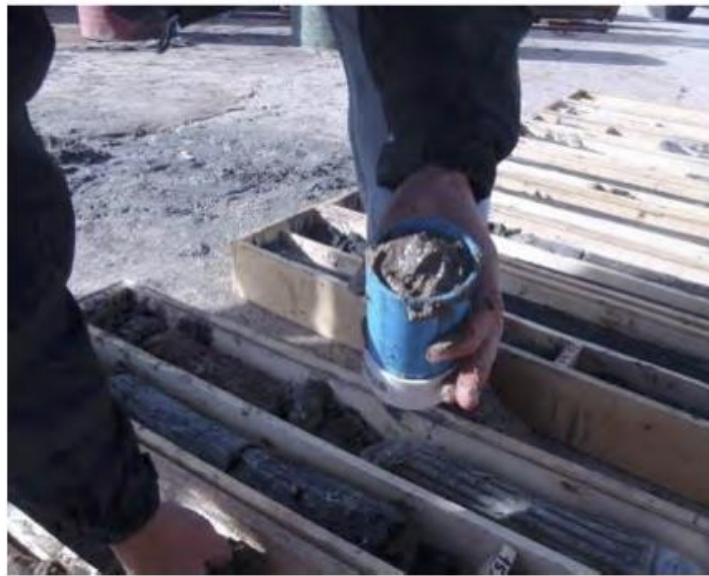
Figure 11.2 Collecting an Undisturbed Sample
