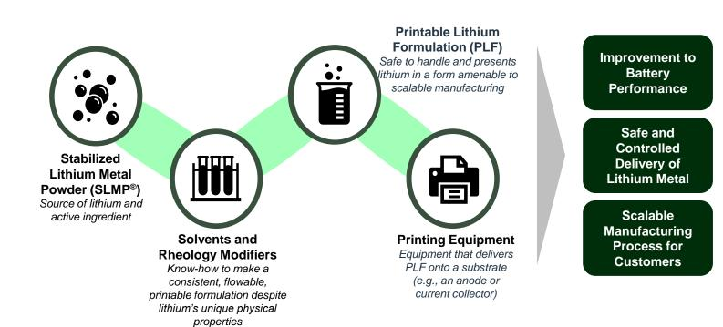
LIOVIX<sup>®</sup>, our Printable Lithium Technology, allows lithium to be deposited onto a substrate in a safe, controlled, scalable manner.
