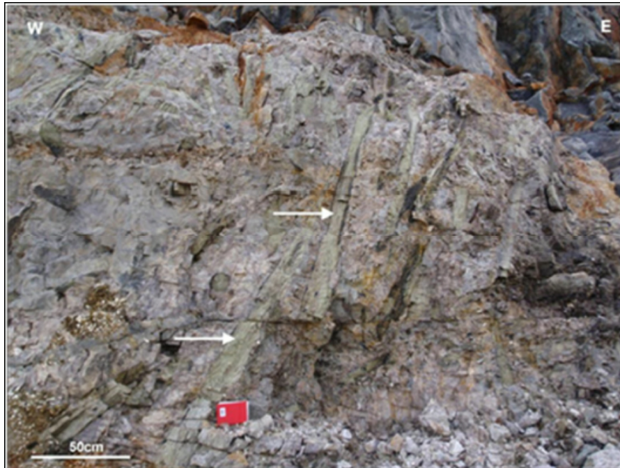
Figure 6-8 - Spodumene crystals in pegmatite (arrowed), Mt Cattlin Pit 1A north wall.
