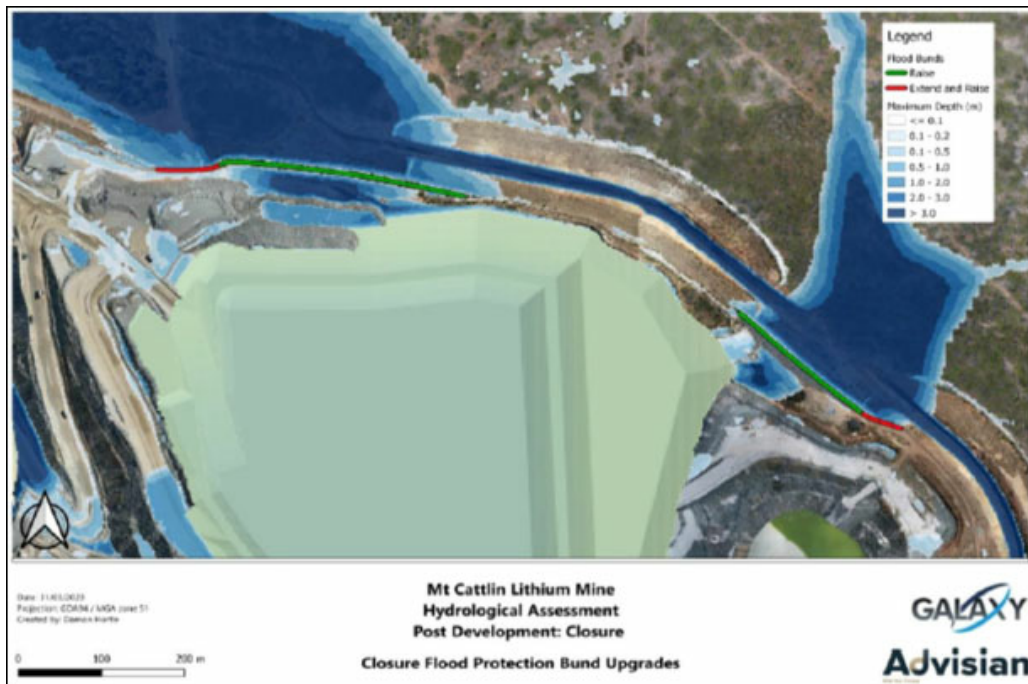
Figure 17-10 - Locations Where Existing Flood Protection Bunds are to be Upgraded at Mine Closure.
