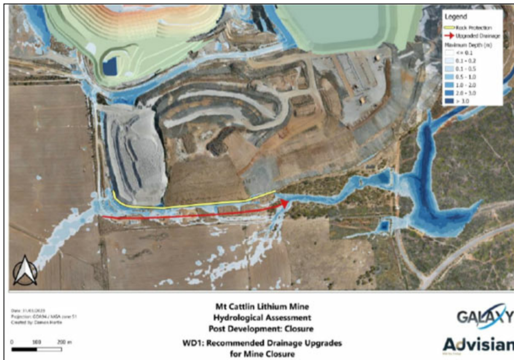
Figure 17-11 - WD1: Recommended Drainage Upgrades for Mine Closure.
