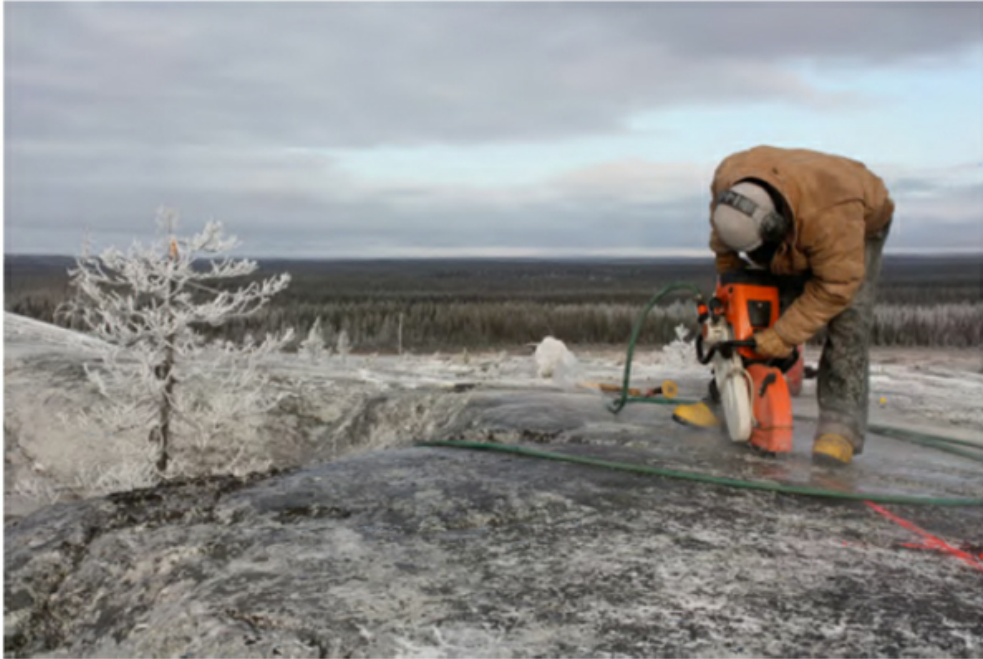
Figure 7-9 - Channel Sampling in 2011 Using a Double-Bladed Circular Saw
