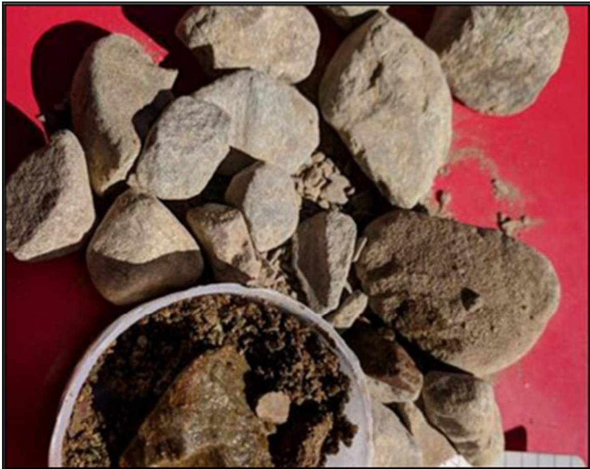
Figure 6-8 - Gravel from CAU16D (264.5-268m) with sub-rounded green quartzites.
