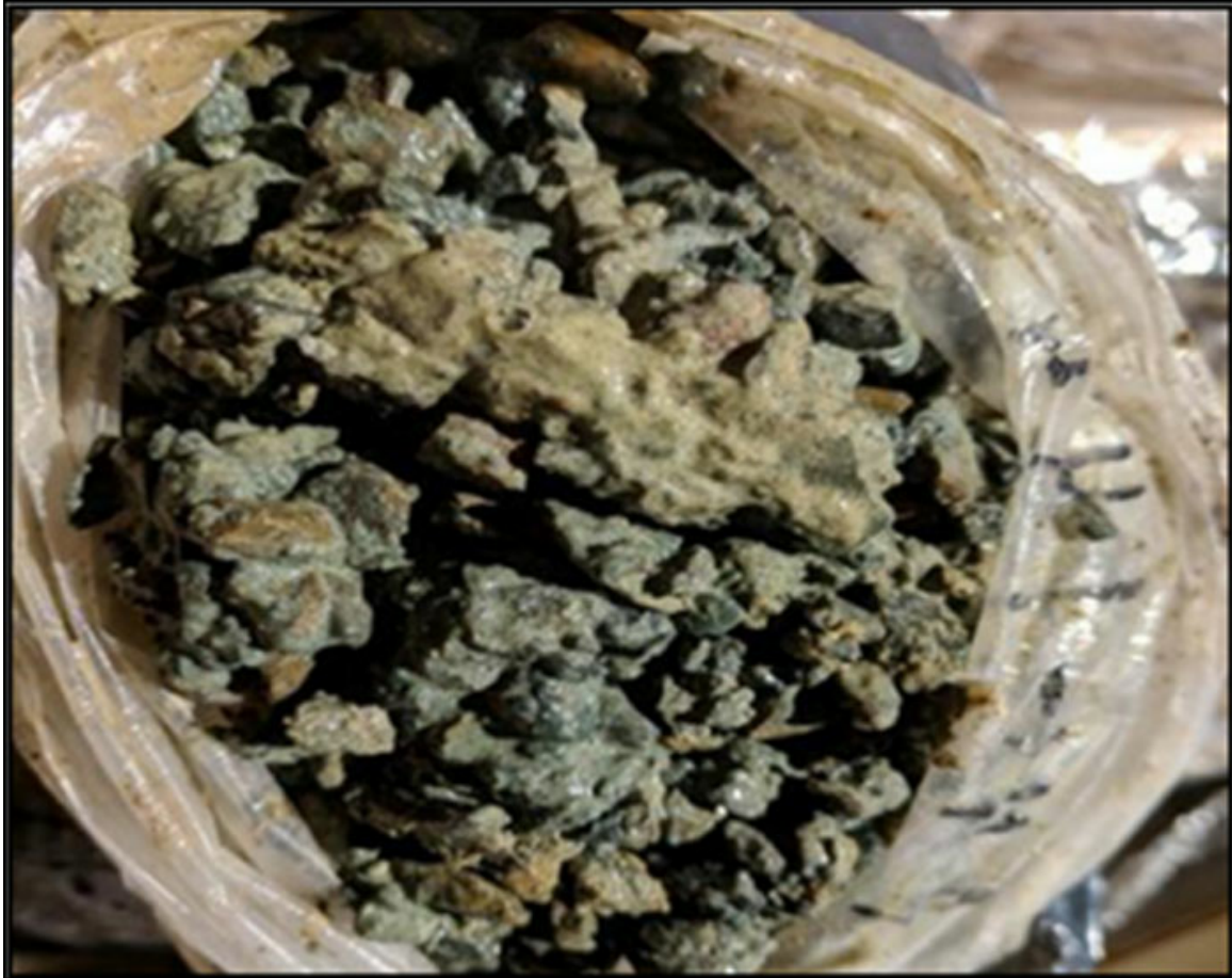
Figure 6-6 - Sandy gravels with some clay from the Archibarca fan (CAU07R).
