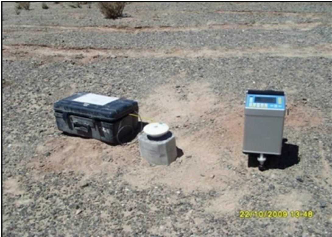
Figure 7-5 - Gravimeter base station.
