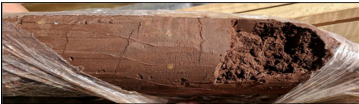
Figure 6-13 - Example of the Clay unit (CAU12D: 177.5-179m).
