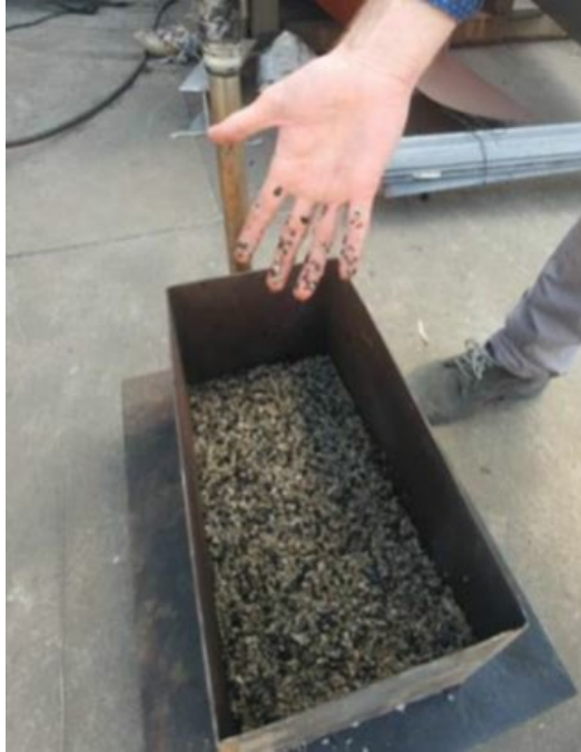
Figure 10-12 ThermoPower Drying Test #2, 80° Discharge Temperature
