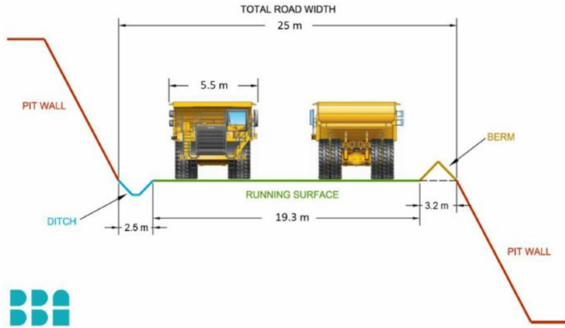
Figure 12-9 Ramp Design
