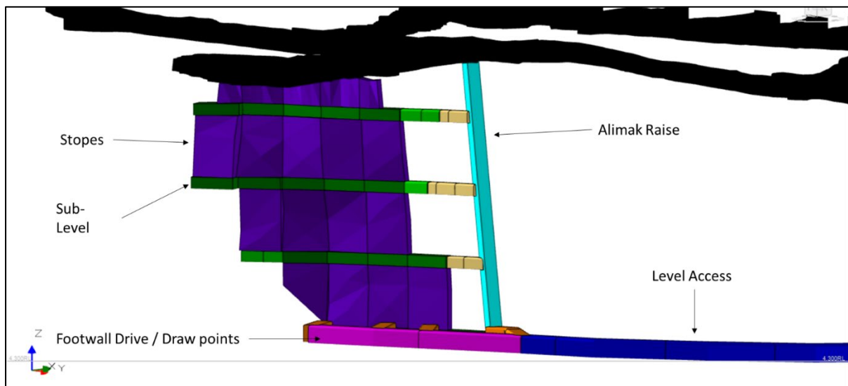
Figure 16-3: Sub-level Open Stopping Captive Access Layout
