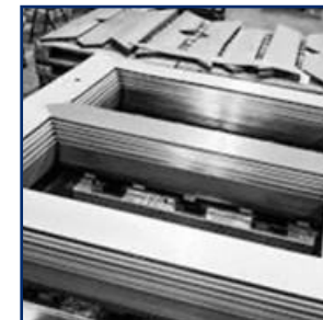
Transformer Core Laminations
