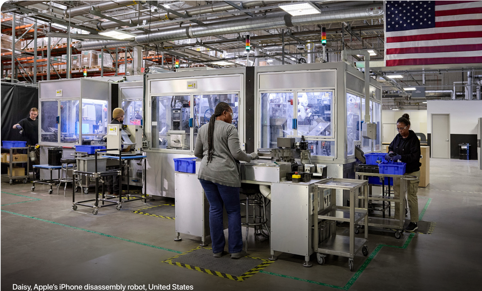
Daisy, Apple's iPhone disassembly robot, United States
